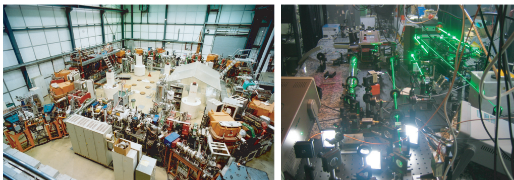
FIGURE 13 Moving clocks go slow: moving lithium atoms in a storage ring (left) read out with lasers (right) confirm the prediction to highest precision (© TSR relativity team at the Max Planck Gesellschaft).
